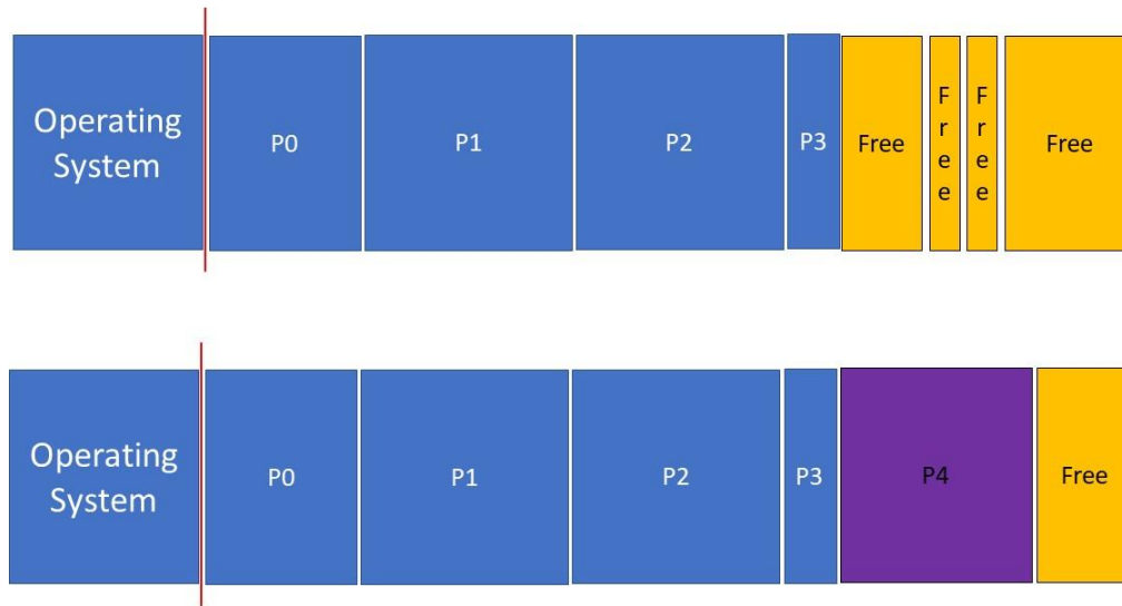
Figure 6.13 continues the ideas from figure 6.12. In the upper diagram, the free memory blocks have been aggregated into one large block (compaction). The lower diagram shows that process P4 can now be loaded into memory.
