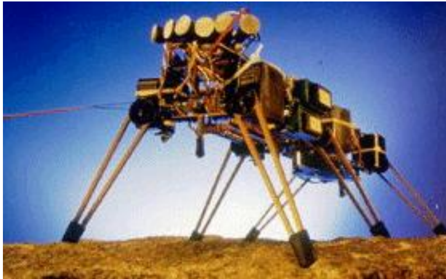
Figure 2. Front view of the MIT AI Lab's Genghis robot. It is a six-legged walking robot with two degrees of freedom per leg.
