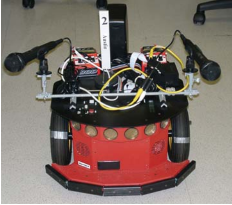
Fig. 4. Pioneer 2DX robot with microphones and amplifiers mounted. Notice how the microphones are mounted on each side of the robot, like ears.
