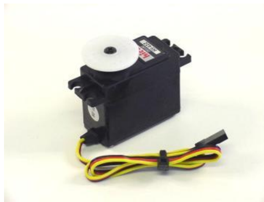
Figure 1. Typical RC servo. The circular white plate on the top of the box is the horn. The horn has a range of rotational motion from 0 to about 225 degrees. Power, control and ground signals enter the servo through the multi-colored cord as seen in the figure.
